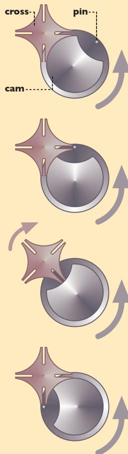
**1** As the wheel rotates, the cross is locked in place by its position against the rotating cam. The curve of the cross fits flushly with the outer circle of the cam ensuring it is unable to move.
